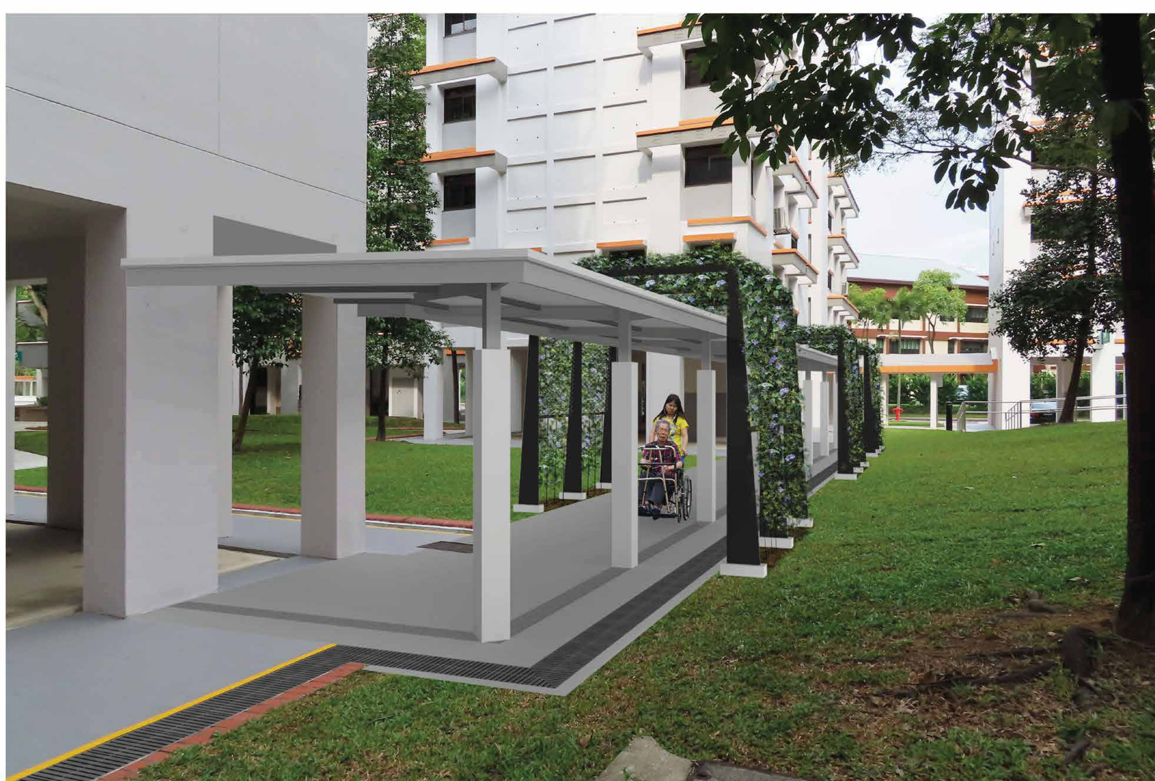
EXAMPLE OF LOW COVERED LINKWAY DESIGN, BETWEEN BLKS 365 & 367A ALL NEW LOW LINKWAYS TO INCORPORATE INTERMITTENT CLIMBER TRELLISES TO INCREASE GREEN FOOTPRINT
